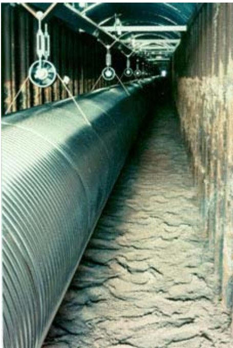
image: evacuated pipe, source: http://www.geo600.uni-hannover.de/geo600/site/photos/Summer_97/tubeintrench.jpg
